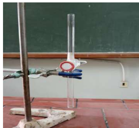
Figure 2: modified Jones reductor
